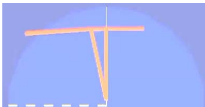
Fig. 7. The third configuration after 1 second — small precession when spin is high
