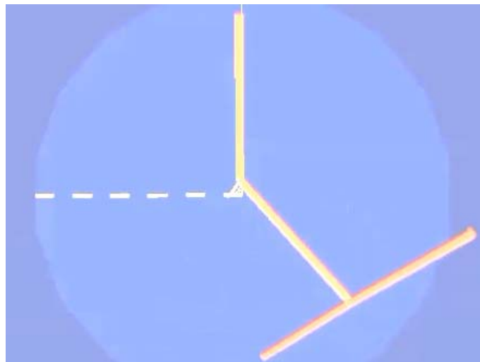
Fig. 5. Configuration after 1 second — large precession when spin is low
